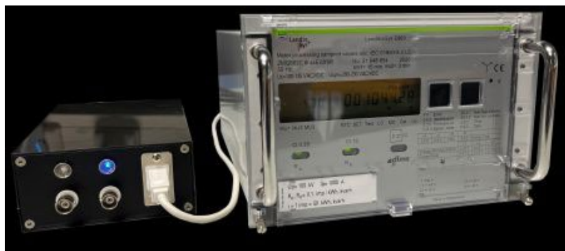
Recently developed SV generator of PTB (left) and commercial energy meter connected via an ethernet cable (right). Credit: PTB
