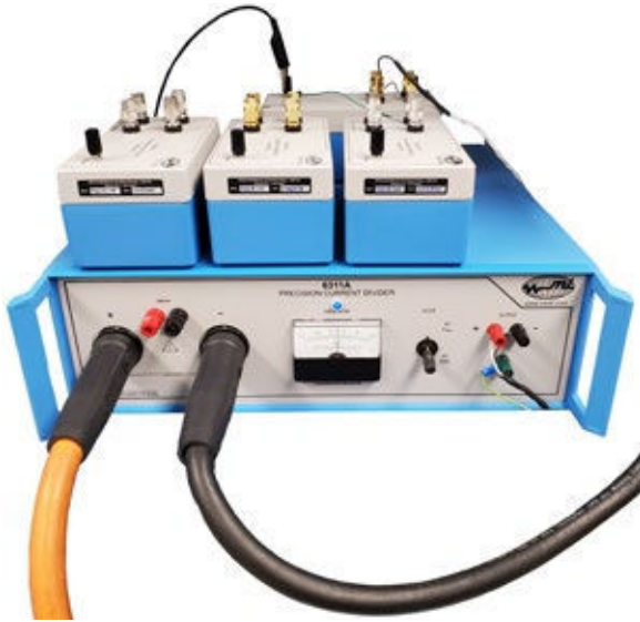
Figure 4. A Measurements International 6311A Precision Current Divider (or DCCT) and four standard resistors.
